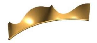
This image shows five morph values applied to a curve with different tangent strengths and rotations. As you can see the derivative field morphing allows very explicit and fine control over the derivative field.
