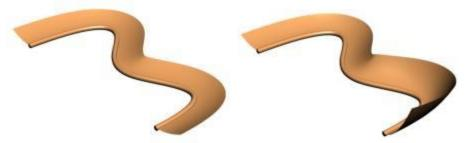
**Radius of Curvature with Constant and Variable Radius**
