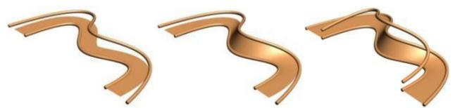
Before and After using a G1 Curve With and Without Specified Tangent Length
